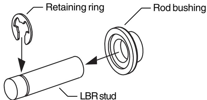
2. Install the long end of the stud assembly into door as shown.
